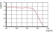
Sensitivity according to the energy necessary to attain a density of 1 above fog
